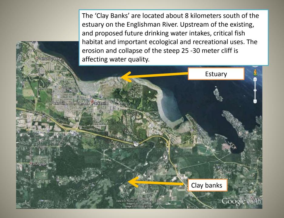
A catastrophic collapse of the clay banks could cause significant problems by temporally damming the river and possibly creating a flash flood.
