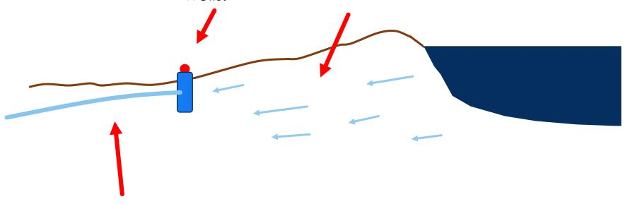
The wells are inter-connected by small diameter syphon pipes, that carry the water downhill under pressure
