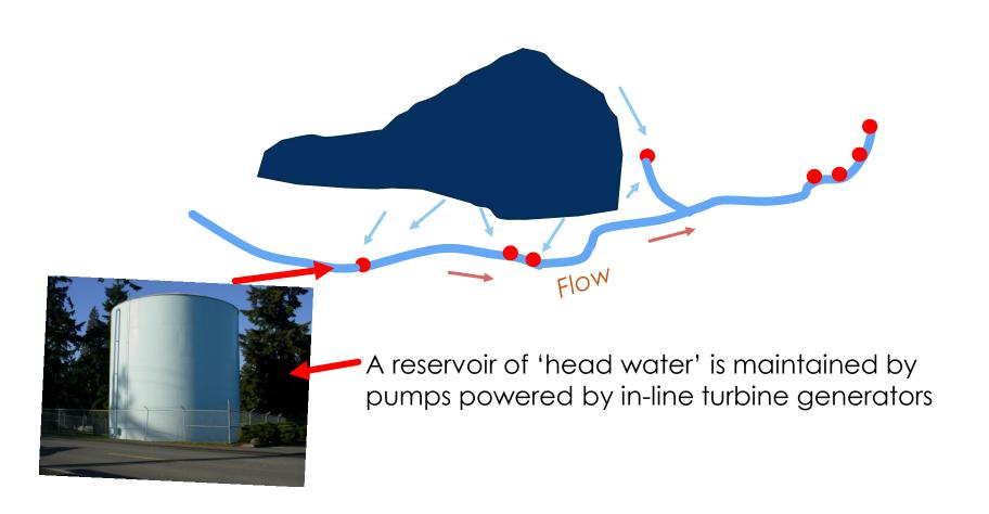
Micro hydro in-line turbines could be installed anywhere in the downhill, pressure side of the supply system.
